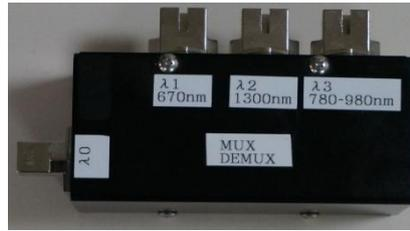
Fig.3. 4-port multiplexer/de-multiplexer (MUX/DEMUX) for GI-POF (Size 90mmx42mmx41mm)
